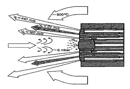
The FLS Swirlax Burner (Fig. 6) applies Pyrojet technology with a license from KHD. The experience in the Holderbank Group is limited.
